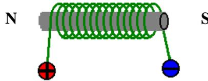
So, we have a conversion of electrical energy to magnetic energy... the force of attraction or repulsion between magnetic poles.
