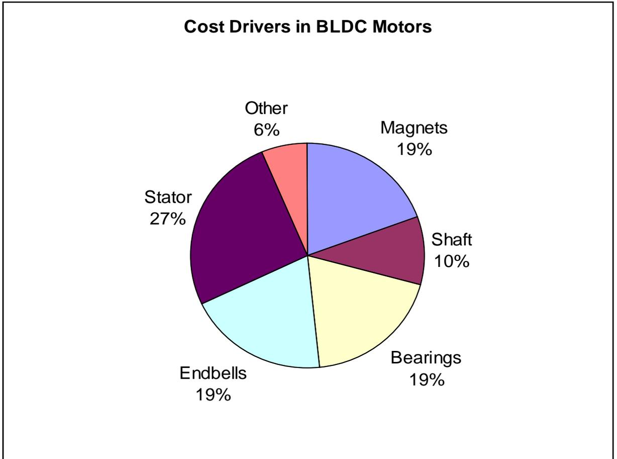
Typically, the cost of the electronics is about as much as the cost of the complete motor. Here again, it may be misleading to generalize but this is a first approximation to give the reader a general idea about the cost and the cost drivers.
