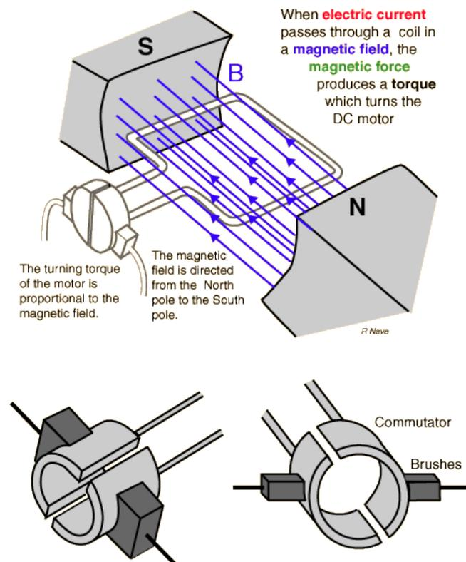
Armature (rotating part or rotor) of a brush type DC motor. The stator is made of a pair or more of permanent magnets or a wound field.
