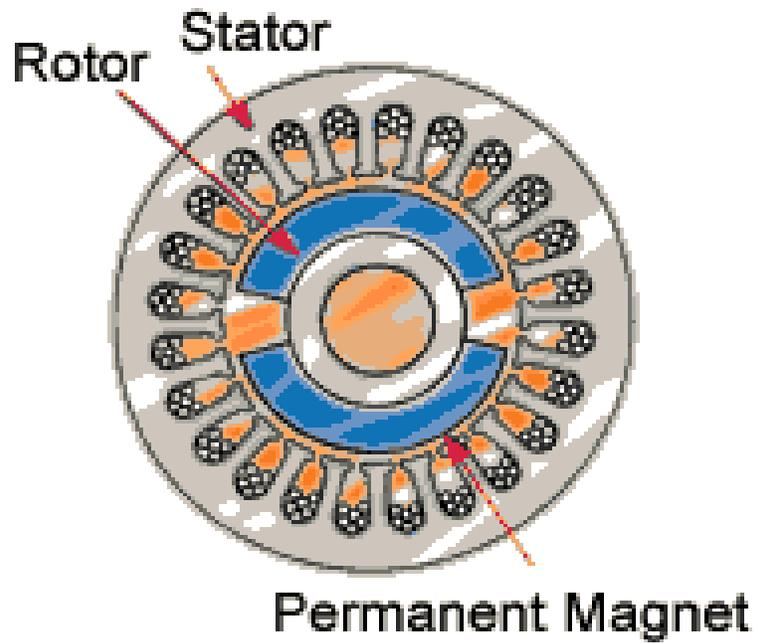
The above is a cross sectional view of a typical brushless DC motor. The permanent magnets are on the inside and on the rotor. The stator is on the outside and has the windings.
