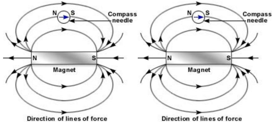
When magnets are brought close to each other, they generate a force of attraction (with adjacent unlike poles) or repulsion (with adjacent like poles). The generation of the mechanical force is fundamental to the way in which all electric motors operate. It can be intuitively seen that to get greater electromagnetic force, the following notions are true:
