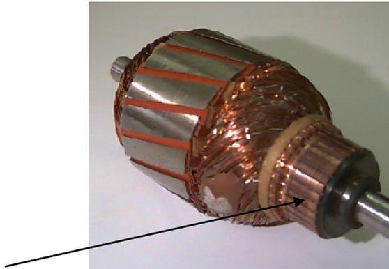
Commutator attached to the armature of a DC motor
