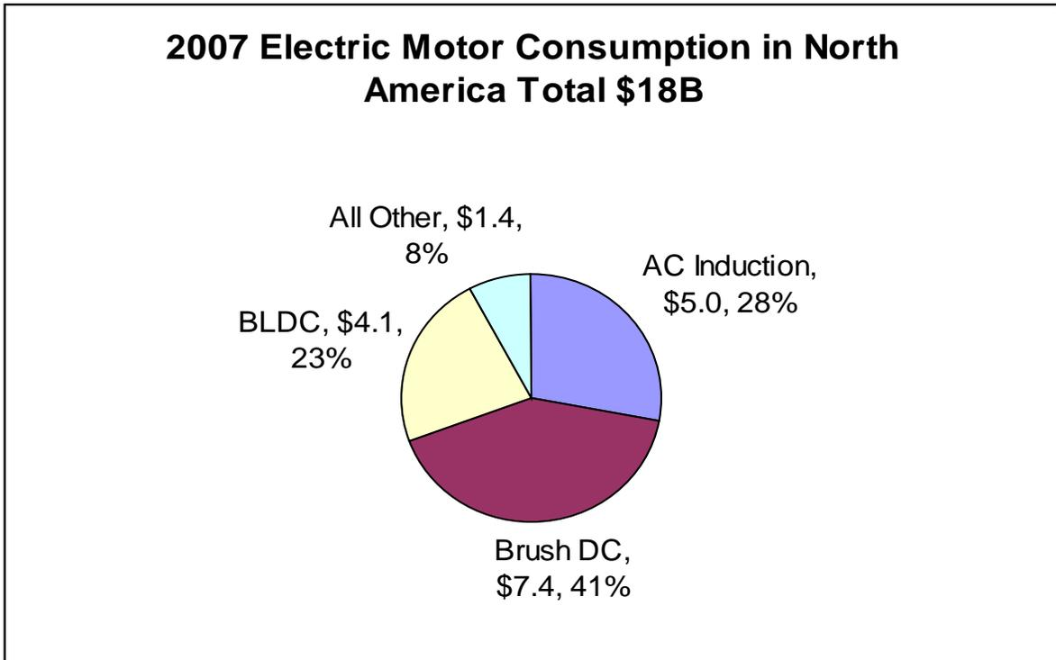
The consumption of electric motors is heavily influenced by the automotive industry and consumer applications. A majority of electric motors used are brush type DC motor, followed by AC induction motors and brushless DC (BLDC) motors. All other category of motors include, AC/DC motors called “Universal” motors used in appliances and stepper motors, used in low end position control applications.
